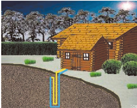
Fig. 2.57 Pond/lake ground source heat pump
