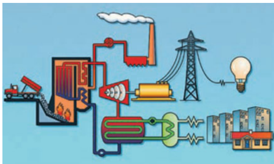
Fig. 2.134 Work schematic for Sysav garbage power plant
