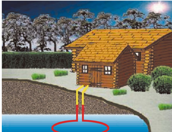
Fig. 2.58 Underground water GSHP
