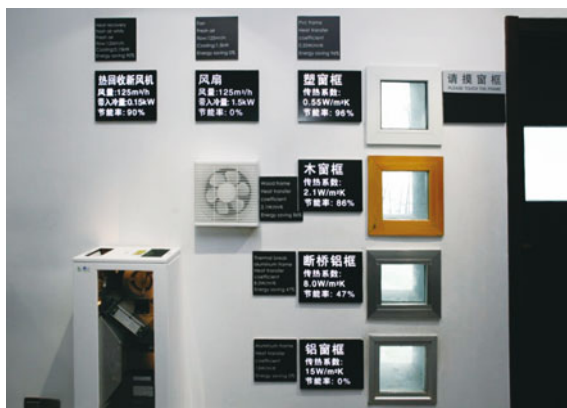
Fig. 3.28 Energy-saving windows inside of the Broad Pavilion
